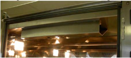
To remove a fan guard: Press as shown at both ends and pull down to unclip from the retaining slots.
